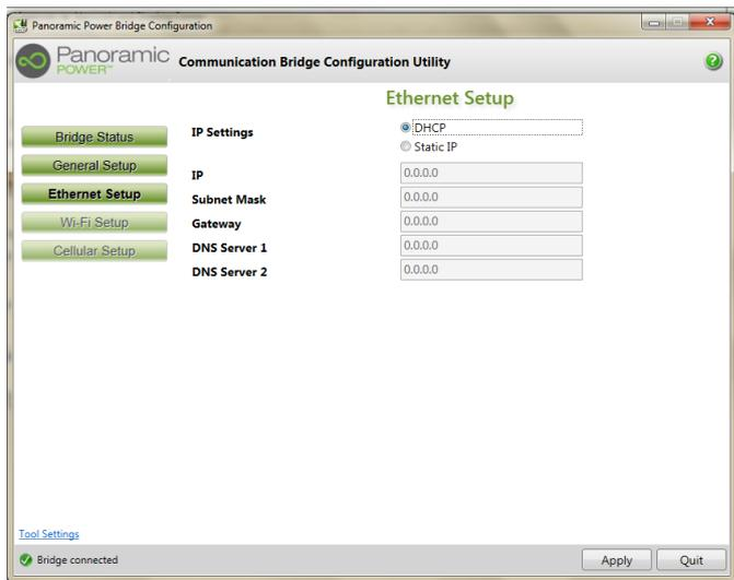
Depending on the method you want to use to define the bridge's IP address, select **DHCP** or **Static IP**.
